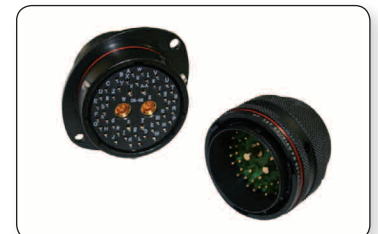
8STA 24-46 specification 251 2 #8 power contacts 4 #16 power contacts 40 #20 signal contacts
